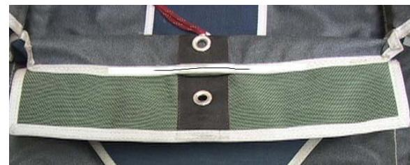
5. Using a medium duty zig-zag sewing machine re-sew main closing flap overlapping the original stitching by 1" on each side.
