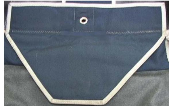
2. Hot cut existing main closing loop retainer just beyond the single needle stitching.
