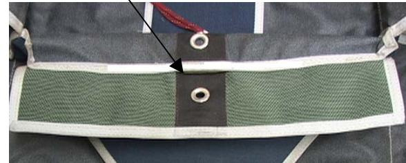
4. Using a medium duty single needle sewing machine sew three rows of stitching one inch past both sides of main closing loop retainer.
