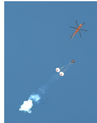
Figure 6. Drogue deploy during Drop Test 3B, courtesy: Boeing
