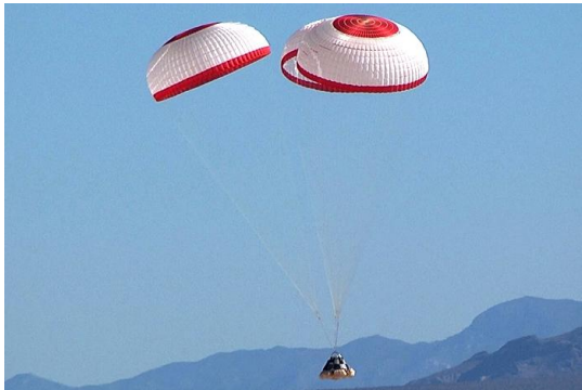
Figure 4. Drop Test 3A prior to landing, courtesy: Boeing.
