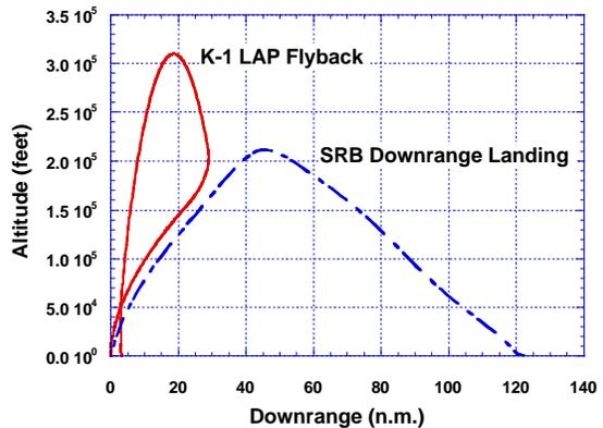
**Figure 5 – K-1 LAP and Space Shuttle SRB Flight Profile Comparison**
