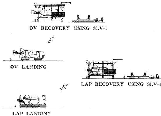
**Figure 6 – LAP and OV Post-Landing Recovery Sequence**
