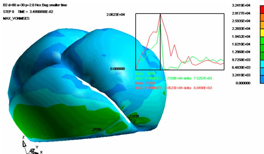
Figure 3. View of Peak Airbag Stress – Outer Shell Portion of Airbag
