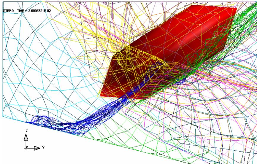
Figure 14. Minimum Lander Clearance – With Spokes – 7.1 inch Clearance
