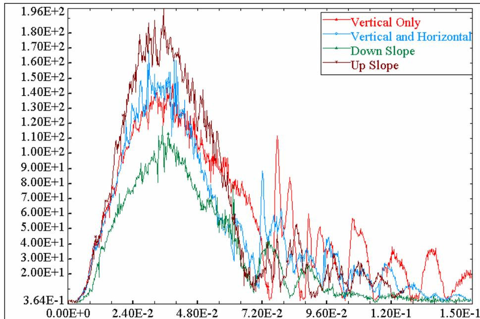
Figure 6. Lander Resultant Acceleration – Four Key Impact Cases
