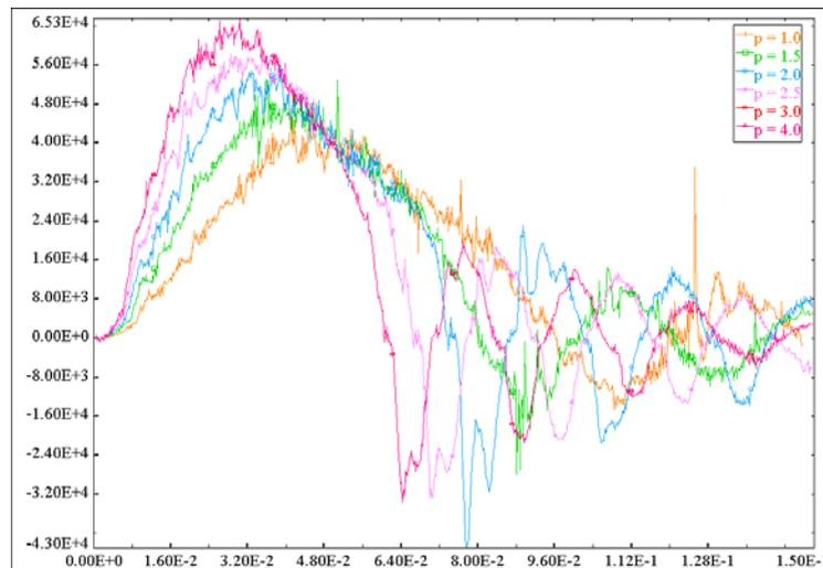
Figure 11. Lander Acceleration Time History – Various Initial Airbag Pressures
