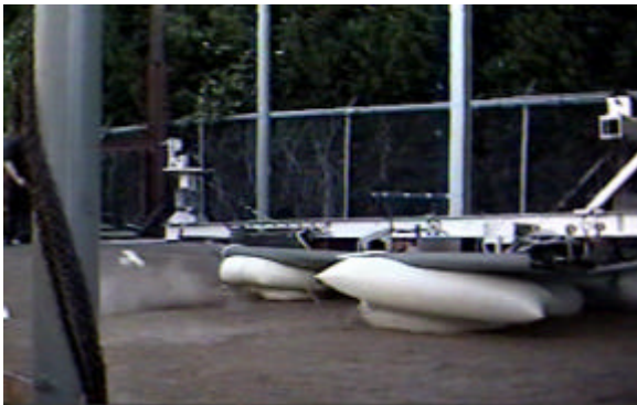
Figure 13 Drop Test Impact Airbag Vent Blocking Against Ground
