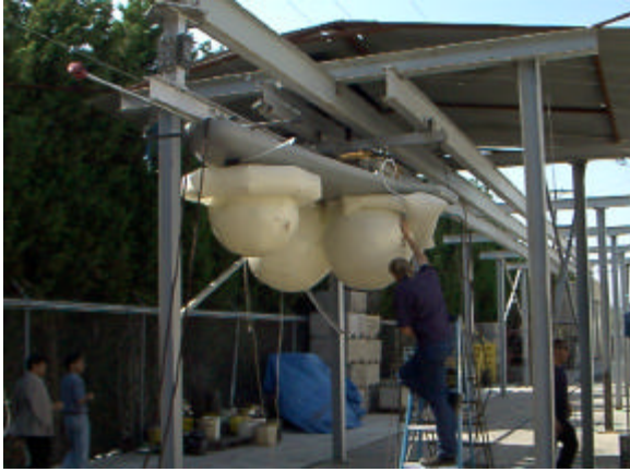
Figure 11 – Airbag Drop Test Facility
