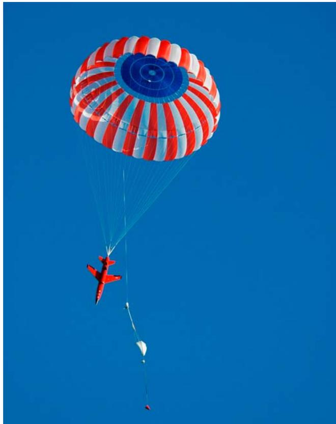
**Figure 12. AFSAT Parachute Recovery System**
