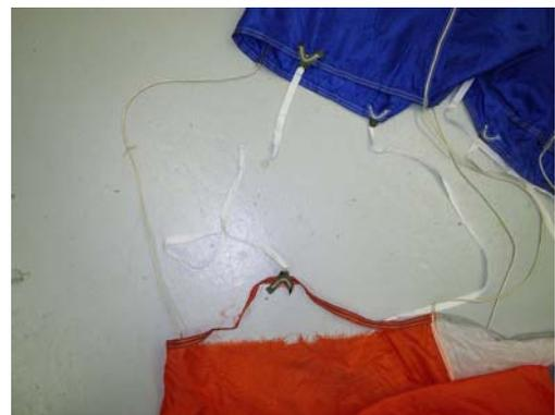
**Figure 6. Typical Vertical Tape Damage**
