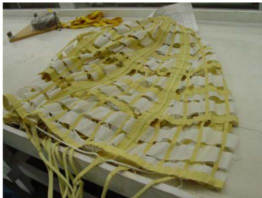
Figure 3. Conical Ribbon Parachute
