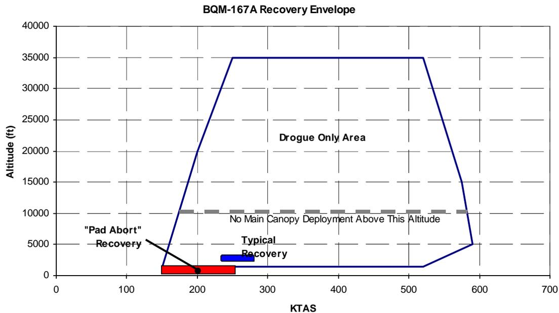
Figure 2. AFSAT Essential Minimum Recovery Envelope
