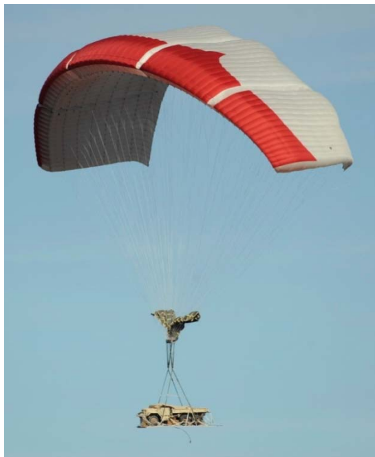
30K MegaFly Drop Test with Deuce and a half truck
