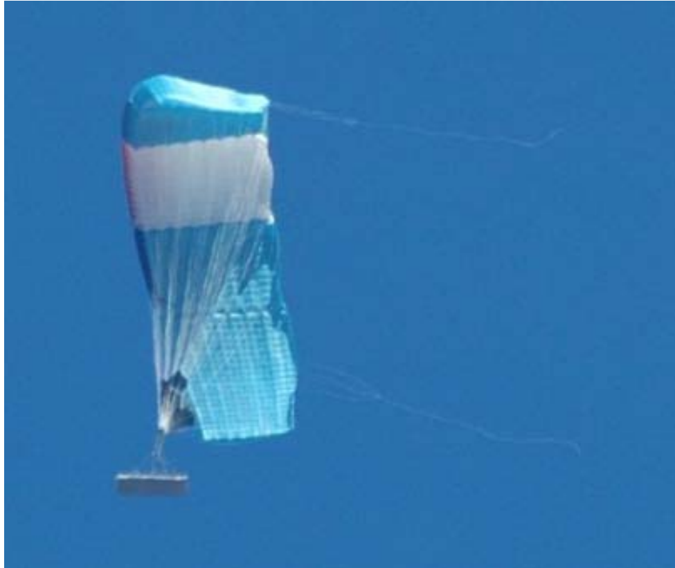
Figure 7 – High Aspect Ratio 42K GigaFly with two broken control lines
