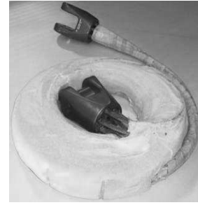
Figure 5. Test Polyurethane mold of 18.2 ft. Drogue Steel Riser
