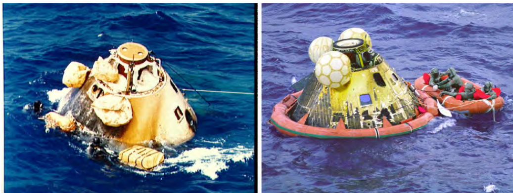
BLOCK I: Apollo 6 Uprighting System & Recovery (Uprighting Bags Deflated)
