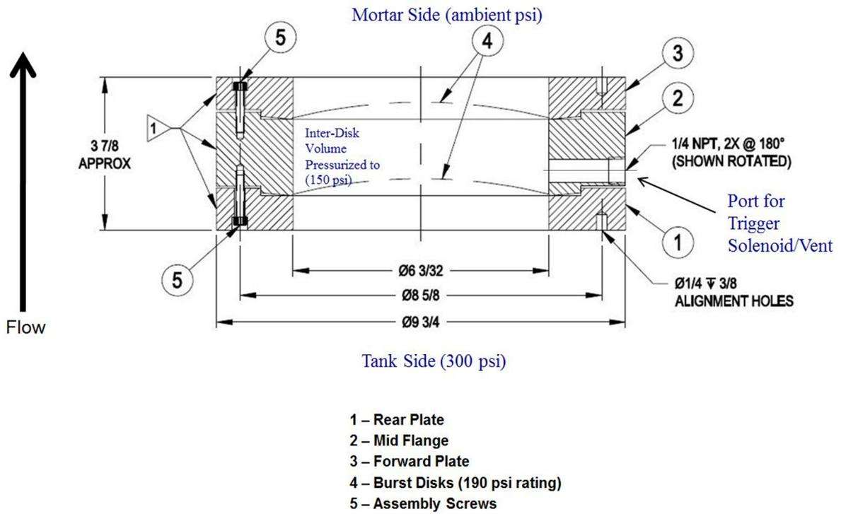
Figure 5. Rupture Disc Assembly
