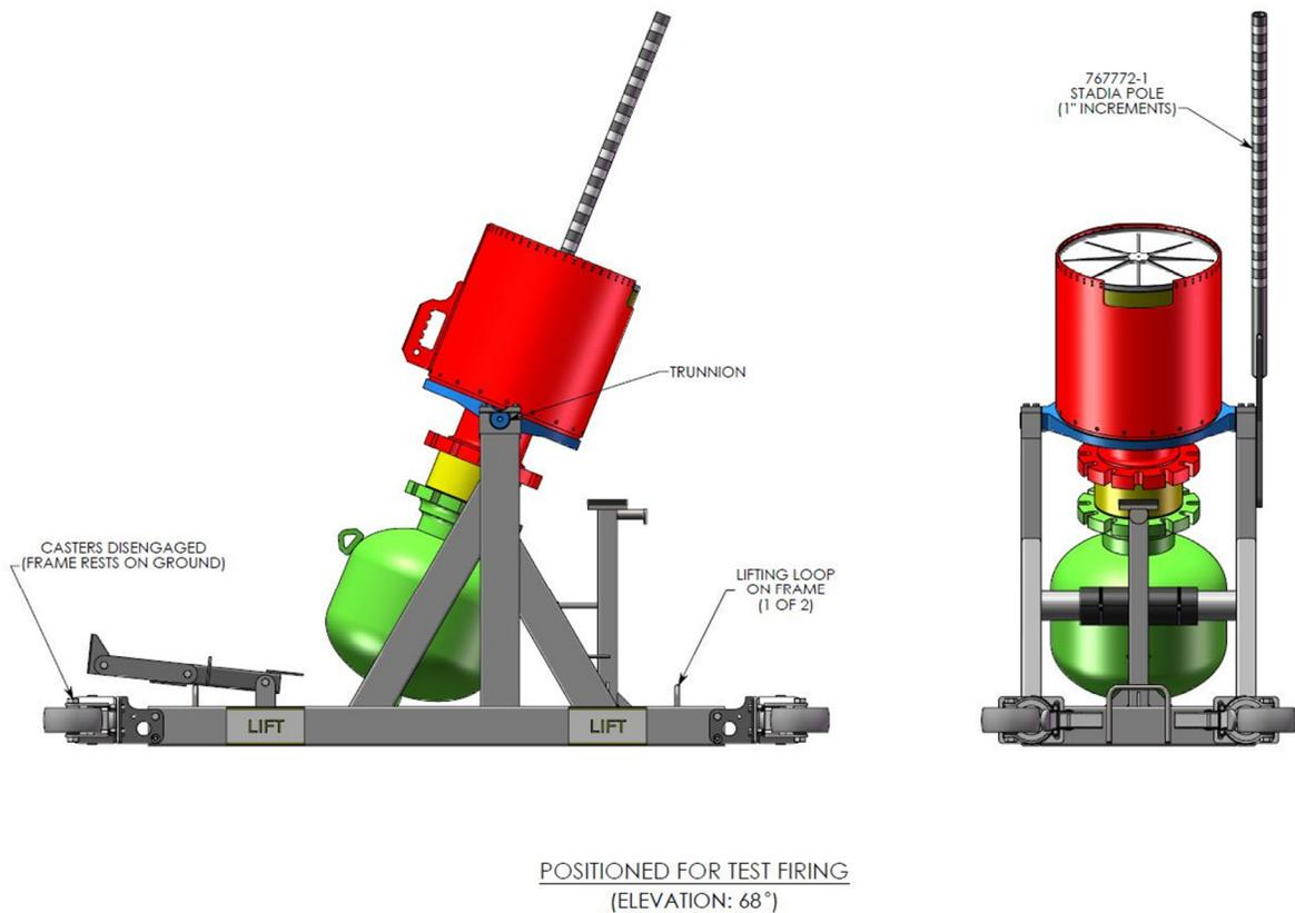
**Figure 4. Pneumatic Mortar in Firing Position**
