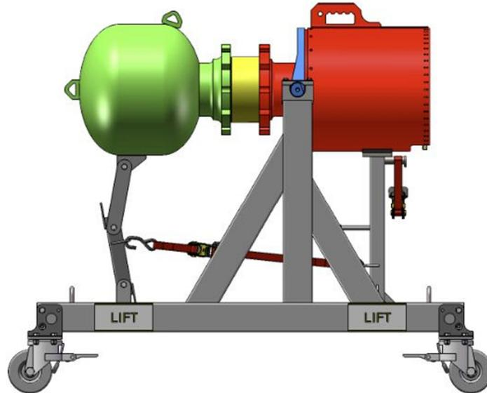
**Figure 3. Mortar Installed In Carriage and in Transportation Position**
