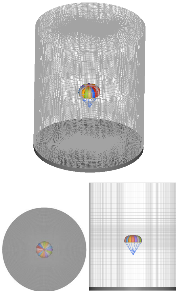
Figure 4. Computational Fluid Mesh with Parachute Structural Model inside.
