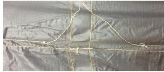
Broken stitches, bottom surface view
