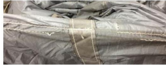
Junction between rib tape and bottom surface tape, view from inside the cell
