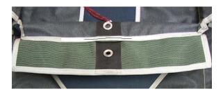
Align main closing loop retainer with the edge.
