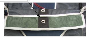
5. Using a medium duty zig–zag sewing machine re-sew main closing flap overlapping the original stitching by 1" on each side.
