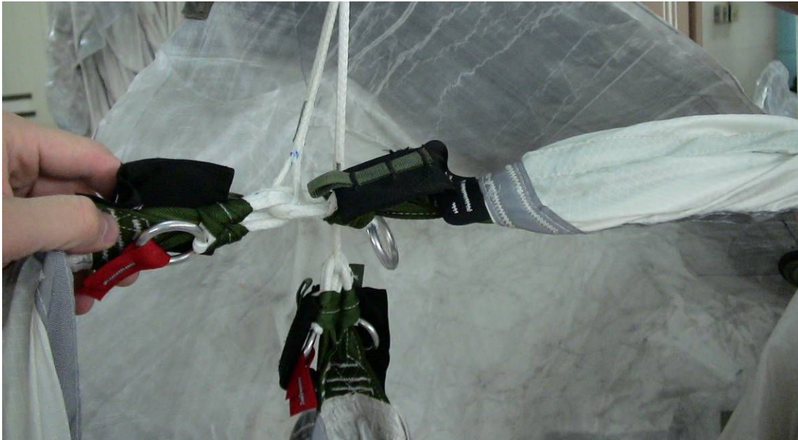
Figure 5: Connecting Cell LAP's Joined Together and to a Suspension Line
