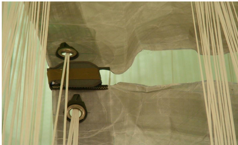
Figure 6: Slider Connection at Spanwise Reinforcement
