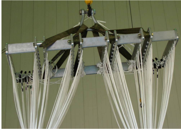
Figure 8: Five Confluence Hardware Sections Assembled w/ Lines Installed
