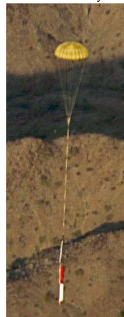
Figure 1. (Left) Plan-form of the full-scale CPAS drogue, and (right) CPAS full-scale drogue flight test with PTV 1 .
