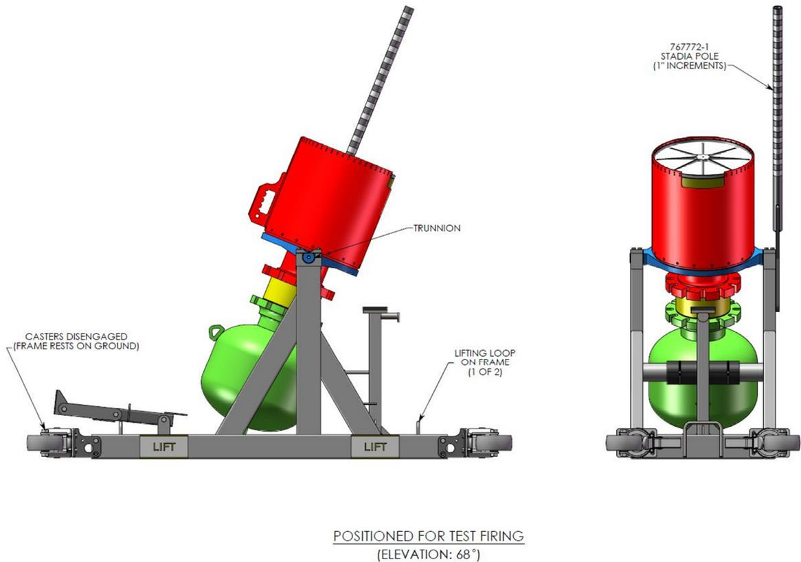
**Figure 4. Pneumatic Mortar in Firing Position**
