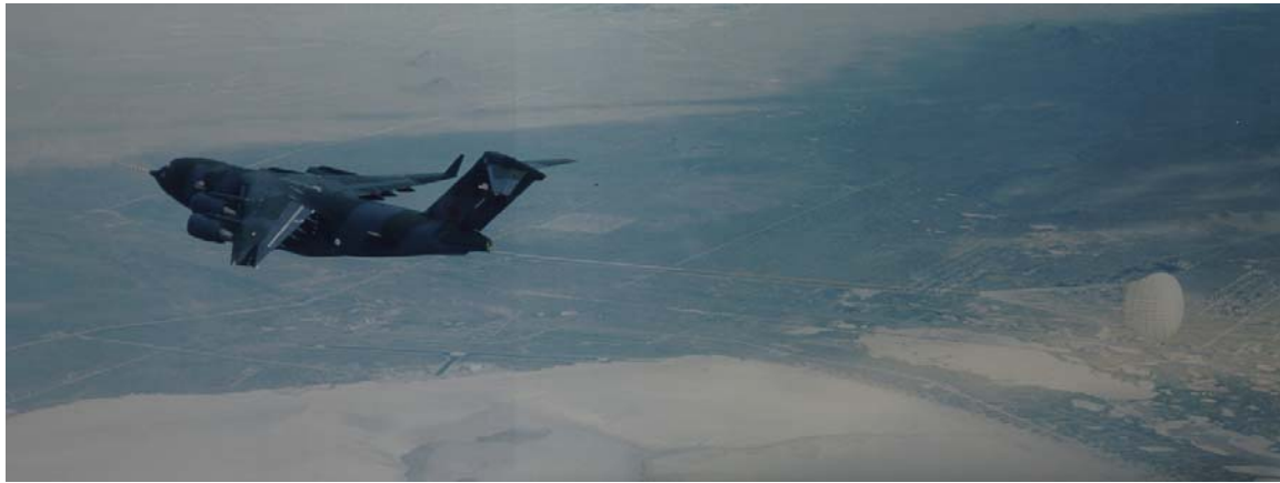
Figure: 17 – C-17 during In-Flight Deployment – Parachute is Reefed to Control Flight Loads
