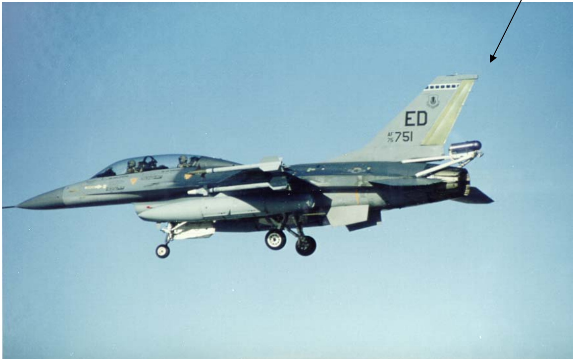
Figure 12 – F-16 Quadrapod for External Installation on a High Performance Aircraft
