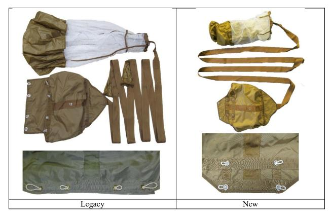
As a result of these improvements, canopy packing procedures and closing of the reserve container are unaffected. The closing sequence of the flaps of the reserve deployment bag is the only change. An addendum to the manual is available to show flap closing sequence.
