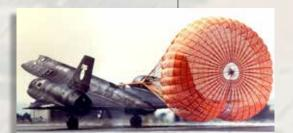
**1963** Landing brake parachute is developed by Irving for SR-71.
