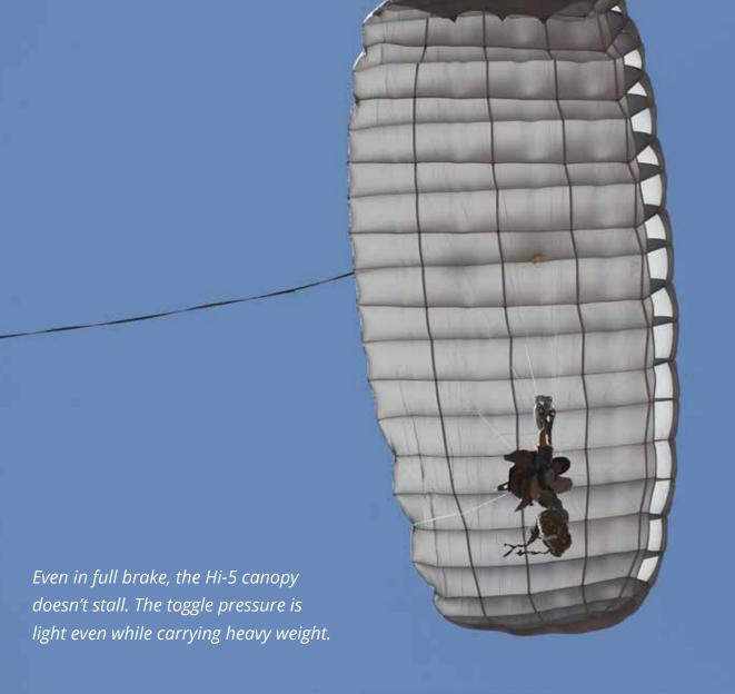
Hi-5 is the most advanced and innovative canopy since the invention of ram air parachutes. It has the reliability and safety of the RA-1 but surpasses its performance in handling, glide ratio, and rapid descent.
