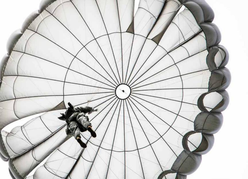
Designed for precision infiltration of airborne forces, MC-6 features the latest in advanced design for steerable troop parachutes. Developed through the Special Operations Forces Tactical Assault Parachute System program, the MC-6 utilizes the same SF-10A canopy that has been in use by U.S. Special Operations.
