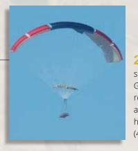
2008 Airborne Systems successfully tests the GigaFly, setting the world record for the largest ramair canopy carrying the heaviest weight ever flown (40,000 lb).
