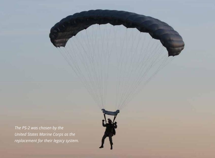
Chosen and type-classified by the United States Marine Corps to replace their legacy multi-mission system, PS-2 is the latest high performance system offered by Airborne Systems. The system features a harness container capable of both bottom-of-container pilot chute and droguefall deployment methods. The drogue system utilizes a new center-of-packmounted drogue release with several key features:
