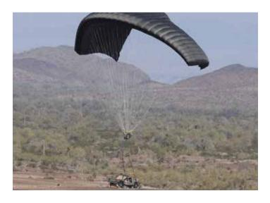
The DragonFly® main canopy boasts the same robust design features as the FireFly® and RazorFly. With 35 cells and a surface area of 332 m<sup>2</sup> (3,570 ft<sup>2</sup>), DragonFly is Airborne Systems' largest commercially available ram air canopy. Riggers with experience on FireFly® or RazorFly will transition with ease to packing and rigging this larger canopy. Only a modest increase in packing area is needed to support DragonFly® rigging.
